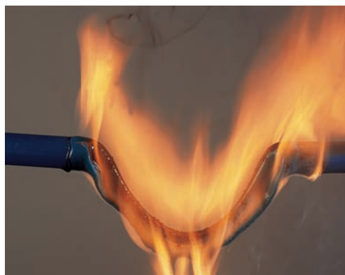
Other Plastics - After torch is removed
