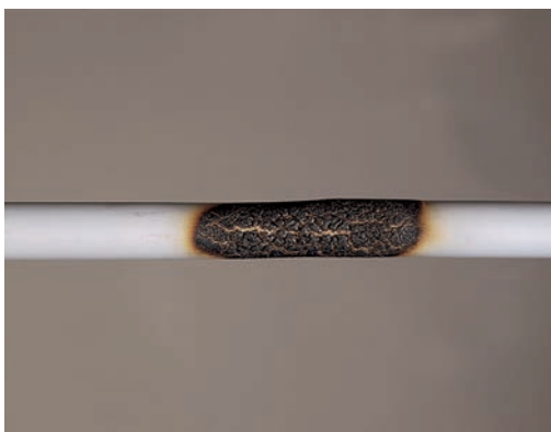
CPVC - After torch is removed
