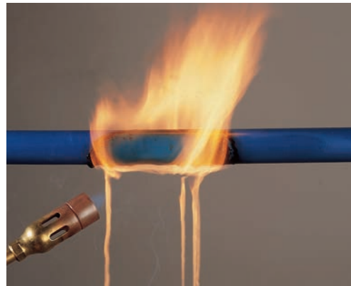
Other Plastics - initially when torch is applied
