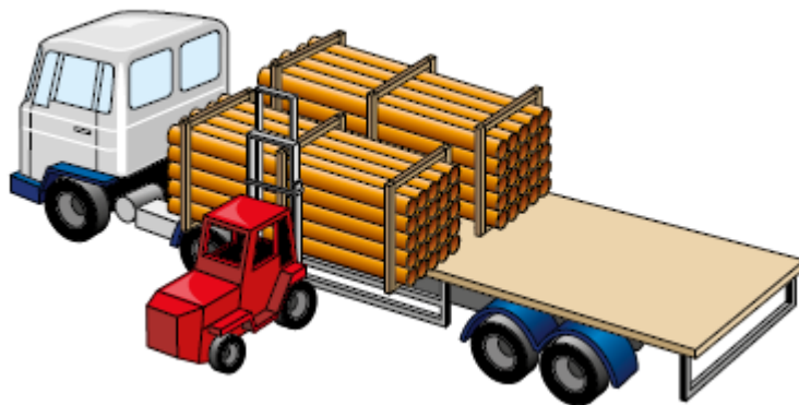
Figure 12: Loading block bundles on to flat bed vehicle
