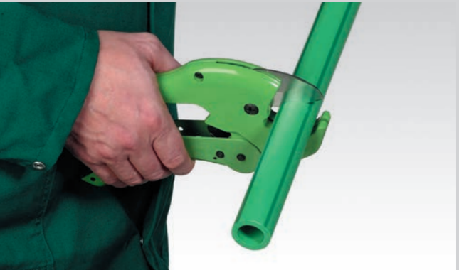
Cutting of the pipe
